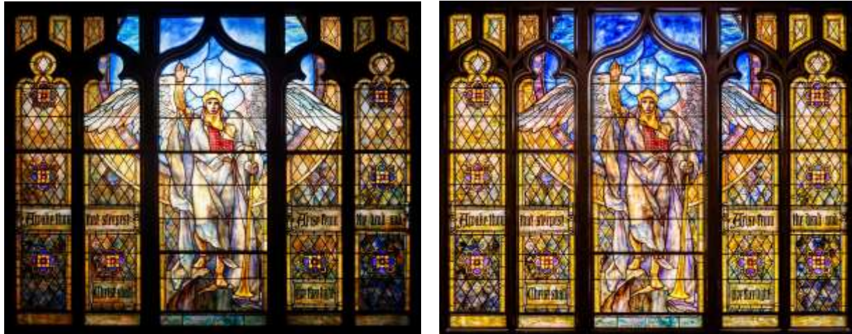
Image 2. Tiffany window illuminated by fluorescent lamps (left) and by LED lamps (right).
